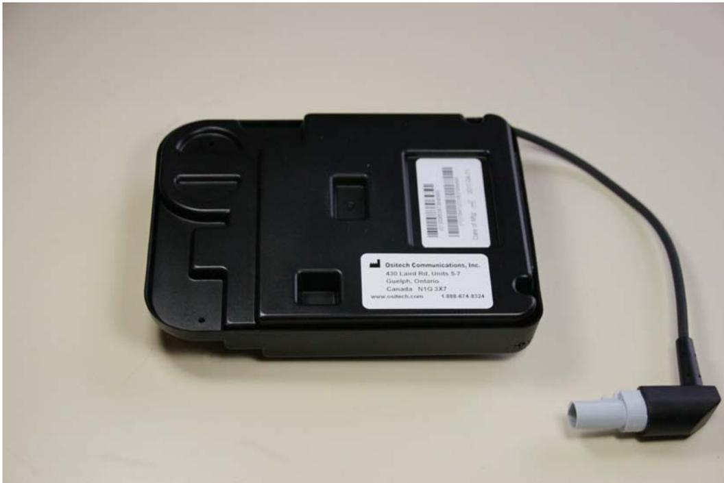
**10. Using one hand, gently separate the clam shell by lifting the bottom side of the clam shell upwards.**
