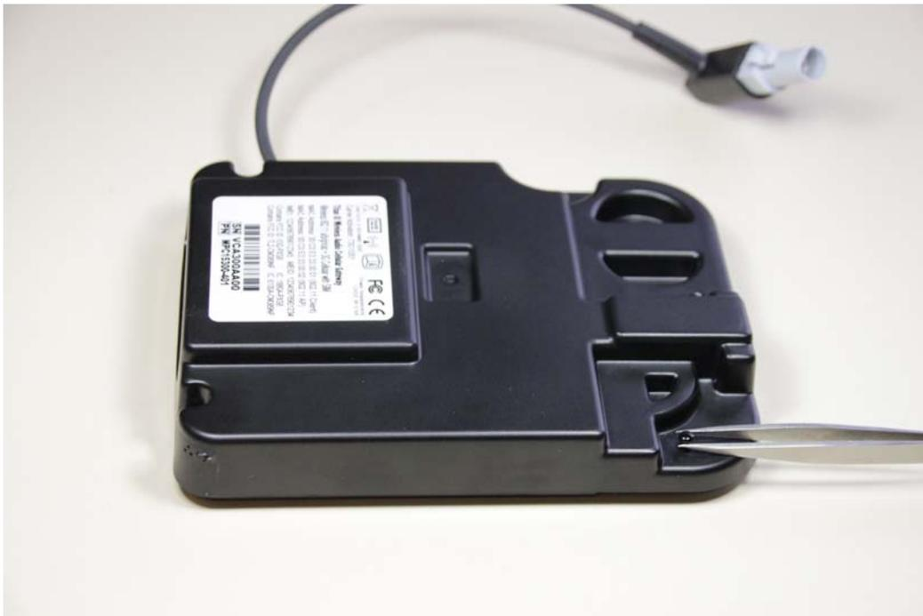
**8. Using the tweezers, remove all four rivets by simply pulling them up. Keep the rivets handy for reuse later to close the clam shell case when done.**
