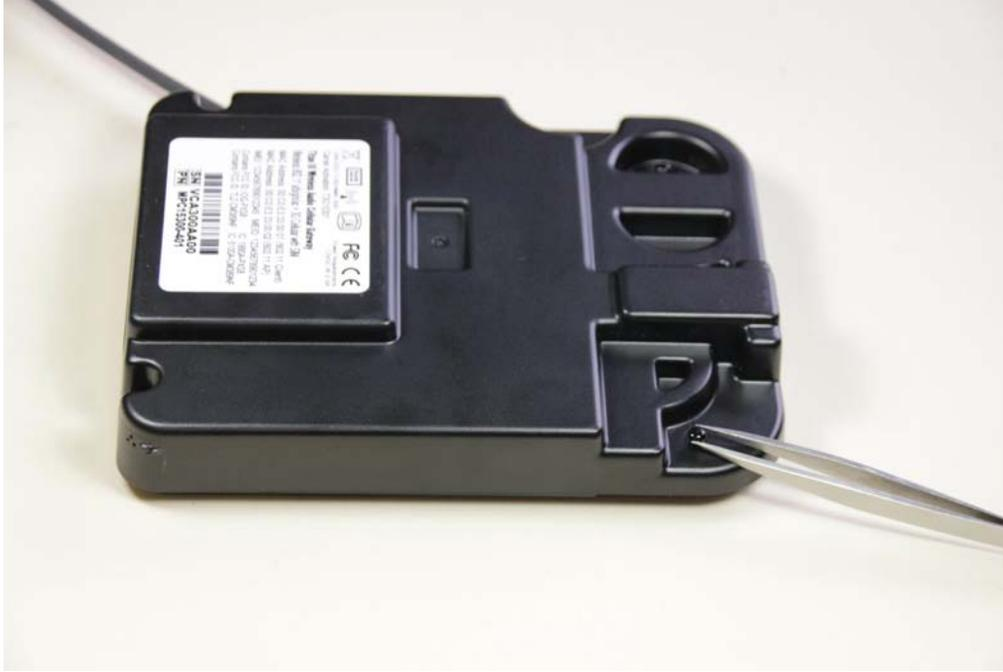
**23. Grasp the Gateway, and examine the plexiglass window. Ensure the SIM Card slot cover is in place, and that the clam shell case is locked and secure.**
