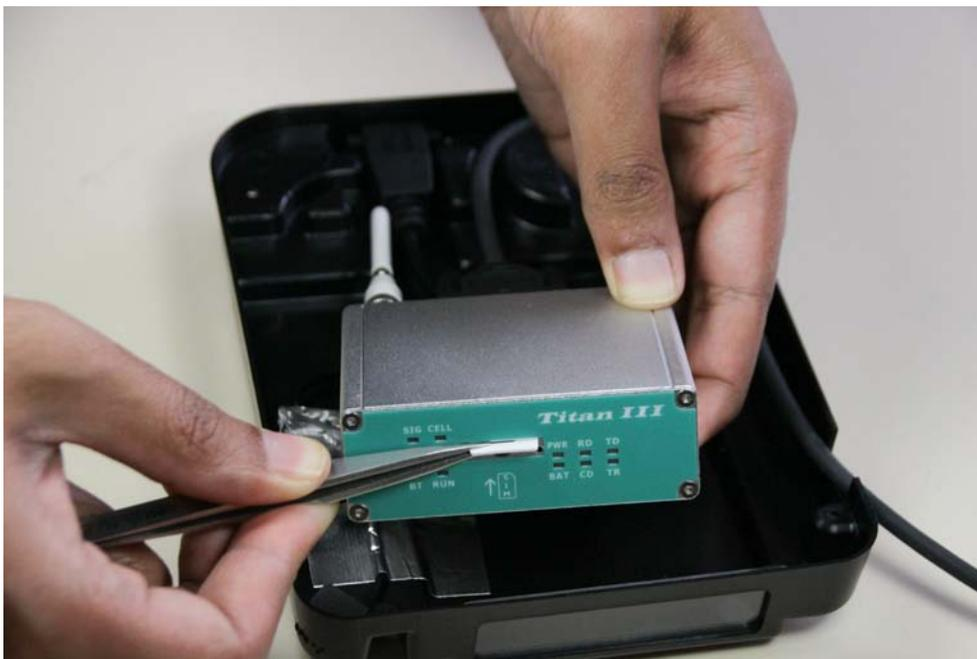
**16. Replace the SIM Card slot cover accordingly.**
