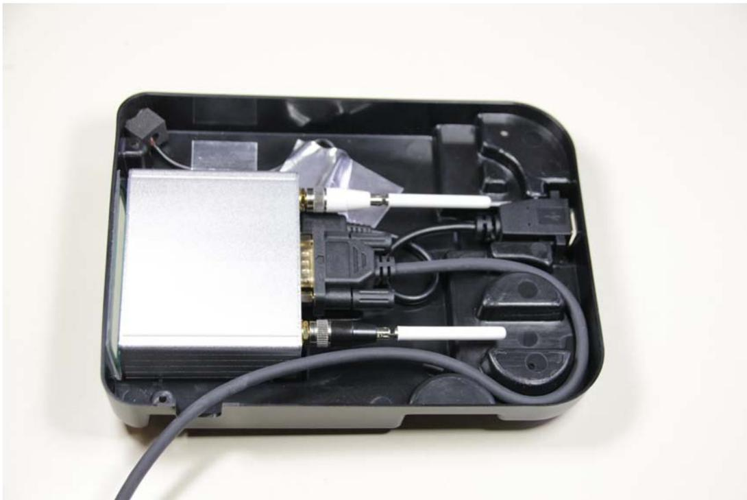
**12. This step can be omitted, if your Ositech Titan III Gateway does not have the Audio feature. Observe the aluminum foil tape. Gently lift the aluminum foil tape to expose the microphone cord below. After you have lifted the aluminum foil tape, unplug the microphone cord from the microphone jack.**
