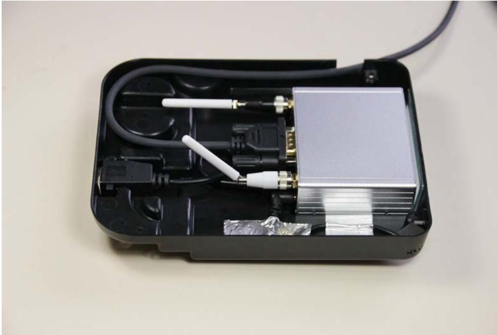
**19. Next, ensure all cables, connectors and antennae are fully seated and secured to the Gateway. Once you have verified all cabling, etc, you will need to route the Hypertronic cable properly. See illustration below.**
