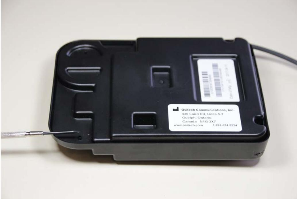
**7. Once all four rivets have been unlocked, invert the clam shell case such that the rivets may be grasped for removal using the tweezers.**
