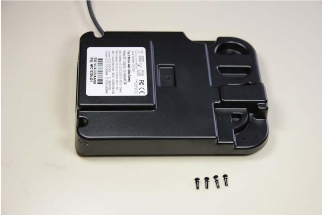
**9. Now that all four rivets have been removed, grasp the clam shell case, and invert the case. The bottom case of the clam shell will now be facing up.**
