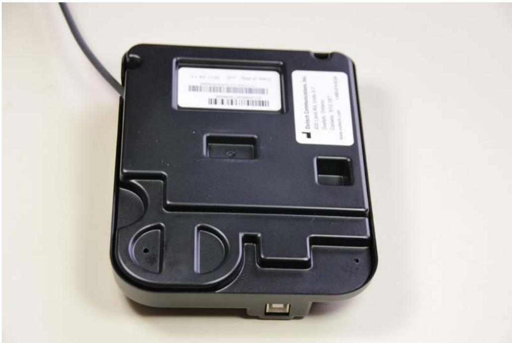
**22. Invert the Gateway, so that the rivets can be reinserted into the clam shell case. Insert all four rivets, and make sure you push them fully into the clam shell case. You may use the tweezers to insert the rivets, and then use the flat head screwdriver to ensure they are fully seated and locked into place. The rivets will automatically lock into place, once they have been fully inserted and seated.**
