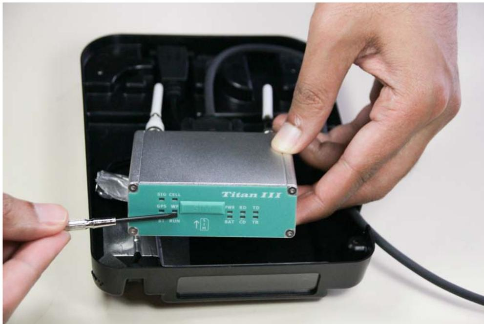
**14. Prepare for SIM Card removal or insertion. To remove an existing SIM Card, simply press the inserted SIM Card until such time you feel the click which unseats the SIM Card. Grasp the SIM Card and remove it straight out. Alternatively, to insert a SIM Card, ensure you have the SIM Card oriented properly. The gold contacts should face upwards, and the notch forward. See illustration below.**
