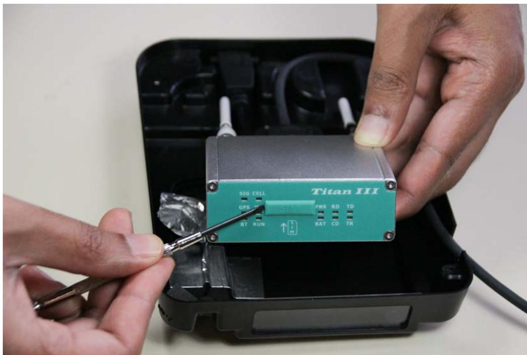
**17. Reconnect the microphone cord into the microphone jack. (For Gateways with Audio feature only)**
