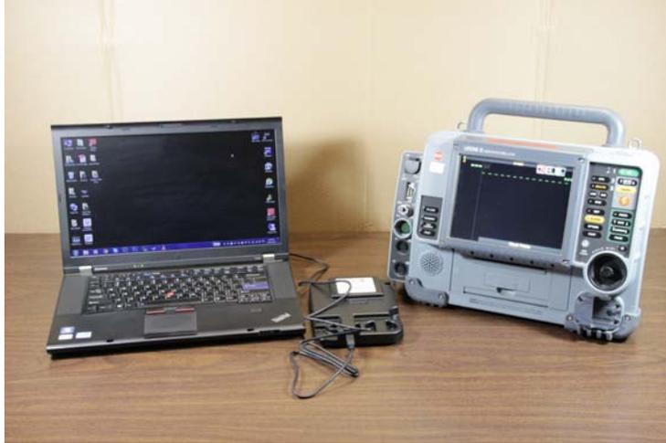
**Connect the Ositech Titan III Gateway to your LIFEPAK device and then power on the LIFEPAK device. Start your computer system, and then connect the USB Cable to the Ositech Titan III Gateway and then insert the other end of the USB cable into any free USB port on your computer system.**
