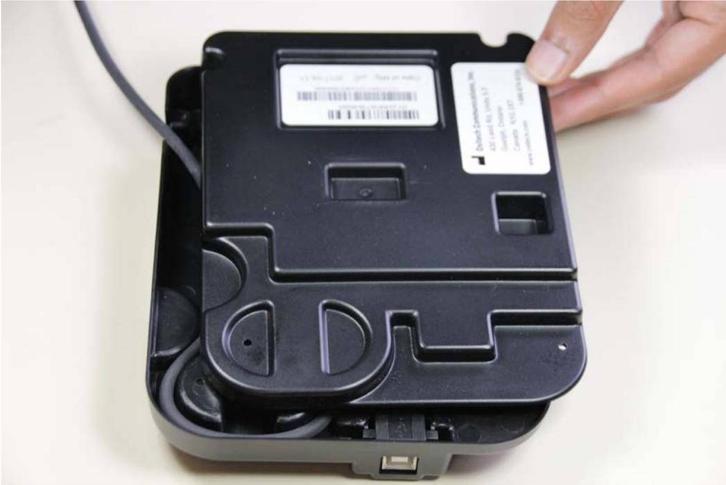
**21. Close the clam shell case. Ensure the Hypertronic cable exiting the Gateway is not being pinched at this time.**
