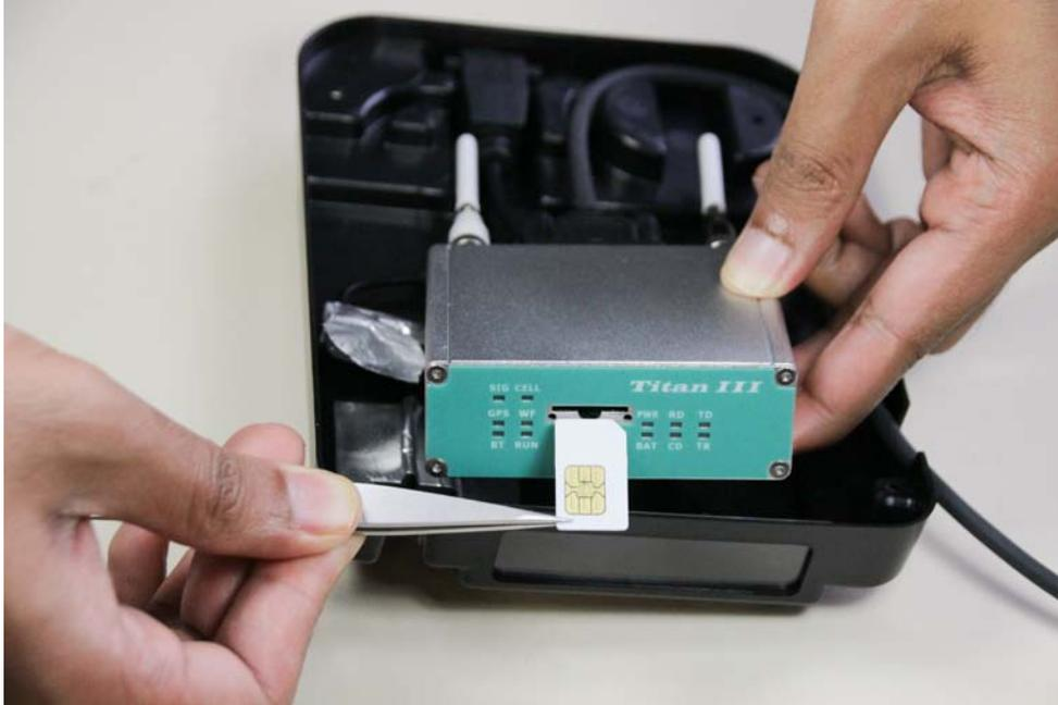
**15. Insert the SIM Card at this point, press and feel for it to click and lock in place. A properly inserted SIM Card will be flush with the face plate and will not stick out.**
