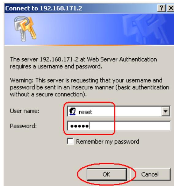
**Once you have logged in using the reset credentials, the Gateway will then perform the reset. At this point, you will need to re-configure your Ositech Titan III Gateway for further use. It is advisable that you import your previously saved configuration, for more ease of use. After a reset, the default username reverts back to “admin”, and the password also reverts back to “admin” (without the quotation marks).**
